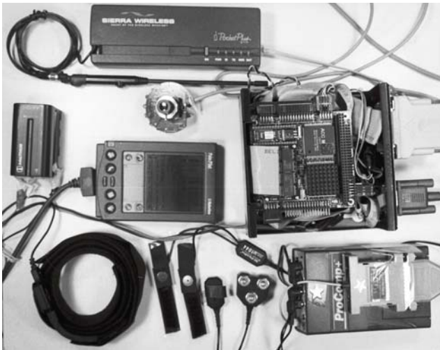
FIGURE 1. Components of the wearable system, clockwise from top: wireless modem, digital camera, wearable computer, sensor monitoring unit, EMG, BVP, GSR, RESP (coiled) PalmPilot interface, battery
