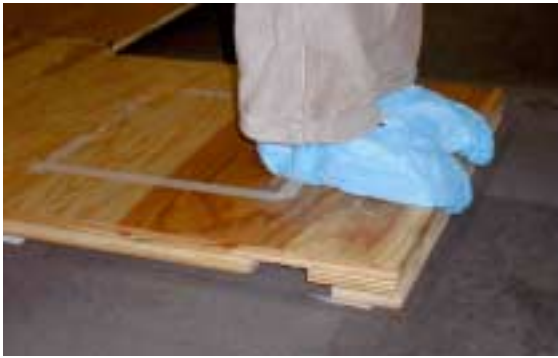
Figure 3. Subject in slippers with toes over 1.5-inch ledge.
