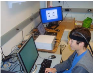
figure 1. fNIRS probe with five near-infrared light sources and one detector.
